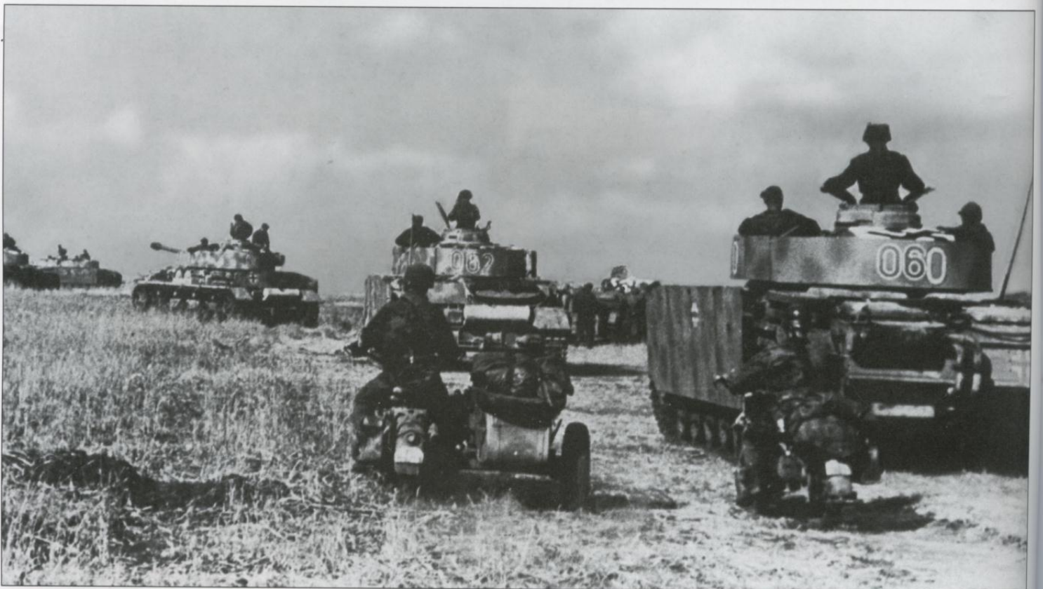
Tanks from an SS division marching in the direction of the front lines. The nearest tank is a Pz.Kpfw.III Ausf.M with a full set of armored side skirts and camouflaged with green spots over the sand background. The tactical number "06" in red with a white outline indicates a staff vehicle. The "0" beside it is white with a thin black outline. In front are the more powerful Pz.Kpfw.IV Ausf.H armed with the 7.5cm L/48 gun.
