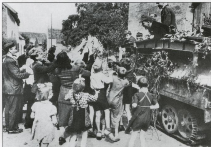
French civilians jostle each other for treats thrown by the SS crew of an Sd.Kfz.251/7 Ausf.D, the Pioniere version of this armored half-track, somewhere in France prior to the Allied invasion in Normandy. The vehicle is liberally covered in foliage as camouflage against roving Allied fighter bombers who had almost complete control of the air. The soldier leaning over the side of the vehicle is wearing a black panzer jacket with an army style piped Totenkopf collar patch and no evident cuffband. His M43 field gray Feldmütze has the SS eagle on the side on a black triangular patch.
