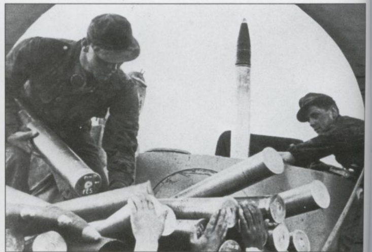
An SS crew replenish their Tiger's ammunition through the loader's hatch in the turret roof. Both men wear the one piece camouflage coveralls with the camouflage field cap. The 8.8cm rounds have colored projectiles for quick identification during battle conditions. The shells with the markings "Pzgr.39" and "FES" are armor piercing and the tip is painted black. The other shells are probably high explosive which were normally carried in equal quantities. The shell casings may also be lacquered steel instead of brass.
