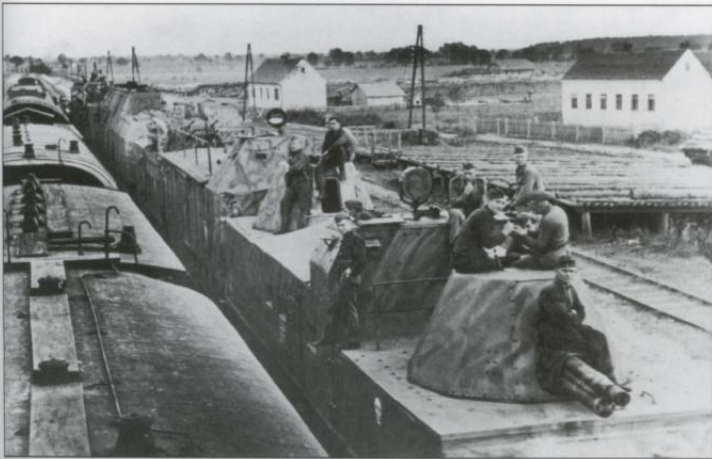
BP42 armored train Nr.64 used to support troops in anti-partisan actions in the Balkans 1943. The nearest wagon is armed with two 10.5cm gun turrets with a raised observation tower between them. The next wagon, the command one, is armed with a 2cm Flakvierling 38 anti-aircraft gun which could also be used against ground targets. The camouflage paint is quite visible on the nearest wagon, green and brown lines painted over the sand background. A white Totenkopf is painted on the side as well.
